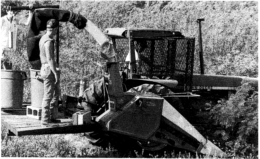
Figure 1. John Deere model 25 silage harvester used to harvest Leucaena . In this figure the 3 point hitch was in the highest position.
